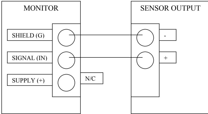
**Figure 6. Connections With Power Supply In Loop**
