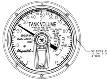
Some Rochester 4” dials have a mounting flange that is secured around the perimeter with several screws. These dials should be replaced by **GSLMH10I00** for remote monitoring.
