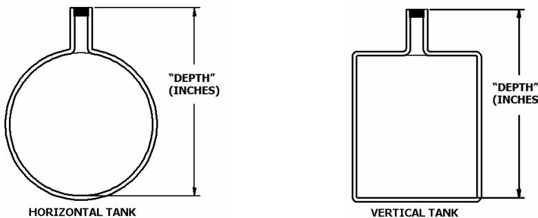
2. Calculate the Cut-Off length for the appropriate Monitor Model Number using the following table and then cut the tape as shown below. **DO NOT cut the tape off if the tank "Depth" is greater than the number that it is being subtracted from.**
