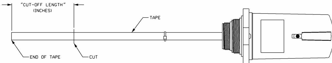
3. Select the O-ring for the tank bung size and install it on the tape. Slide the float, then the anchor on the tape. Align the end of the anchor flush with the end of the tape and tighten the anchor screws to a minimum of 10 in-lbs.
