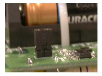
• Once the Disable Jumper is removed from the PCA of the Monitor, the Controller should flicker LED light to indicate that it successfully received a Monitor transmission.
