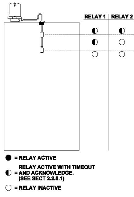
Figure 2: Dual High Alarm Operation
