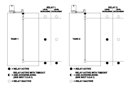
Figure 3: High-Low Alarm Operation
