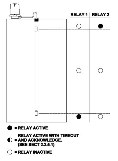
Figure 4: Midrange Alarm (Dual Float) Operation
