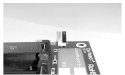
Figure 2. Disable Jumper in enable position
