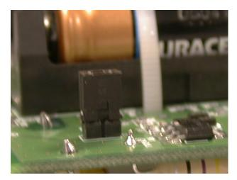
Once the Disable Jumper is removed from the PCA of the Monitor, the Controller should flicker LED light to indicate that it successfully received a Monitor transmission.
